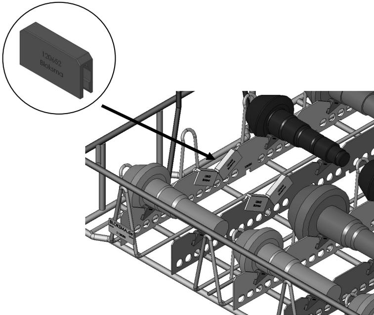
Delicate parts lie on plastic elements. These can be clipped onto the receiving strip.
