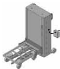
detachable control panel
